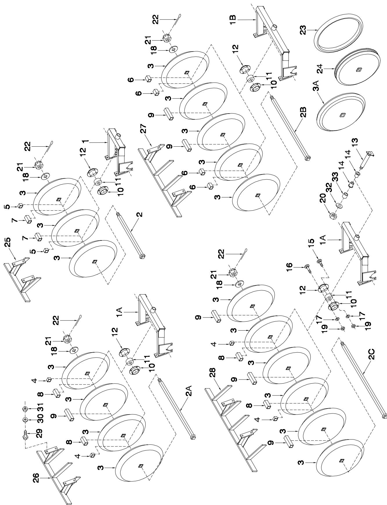
**Packer Gangs - 10" Spacing - 4.5" Steel or Rubber - Prior to September 2008**
