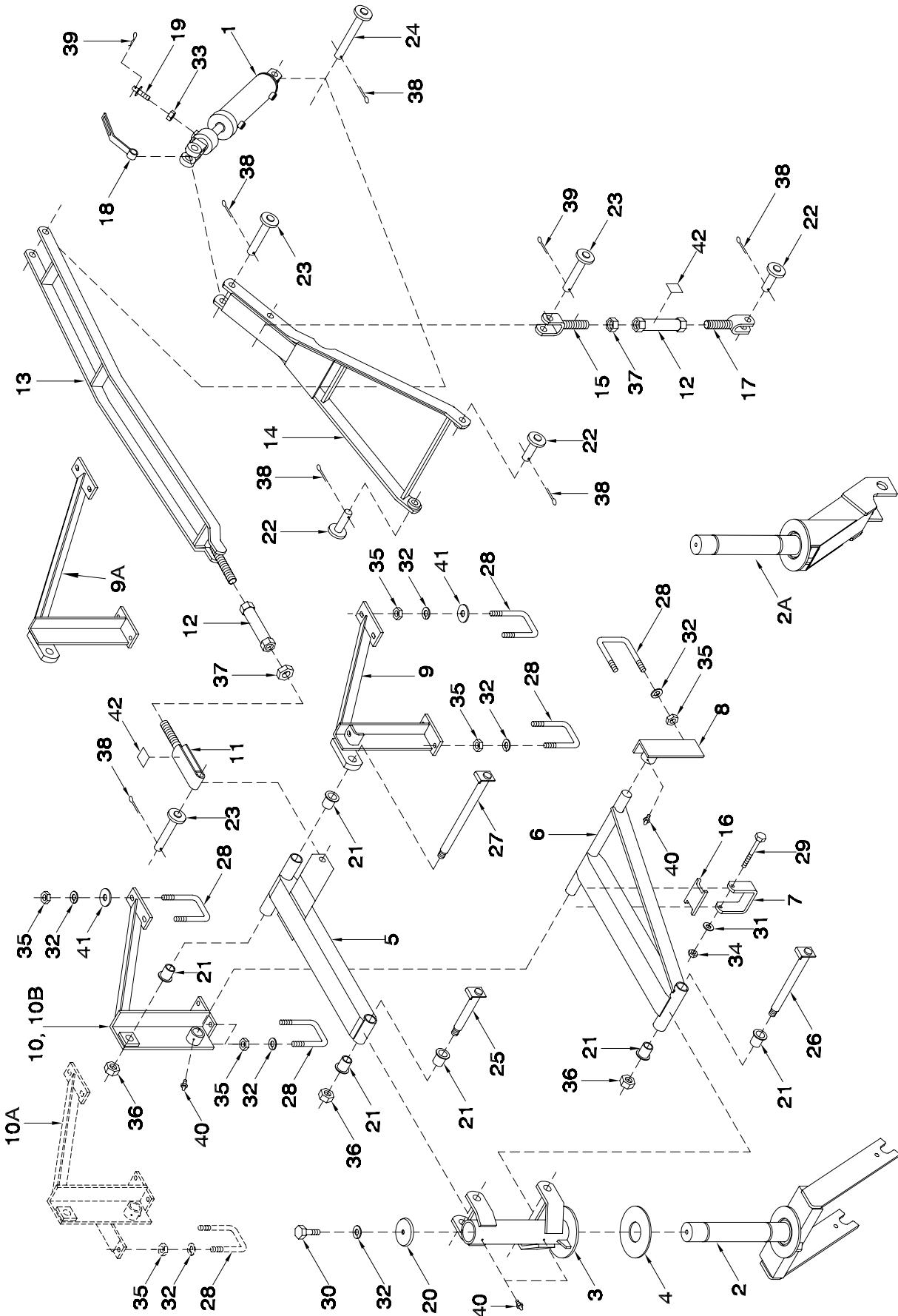
**Depth Control Linkage - Left Gauge Wheel 34 ft, 49 ft Inner Wing & 60 ft Outer Wing**
